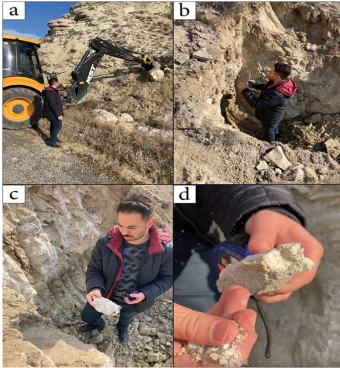
Figure 5. (a) A view from the exploration pit opening. (b) A view from Research Pit-1. (c) A view from Research Pit-2. (d) An image of the altered gypsum sample, which disperses even in hand [11].
